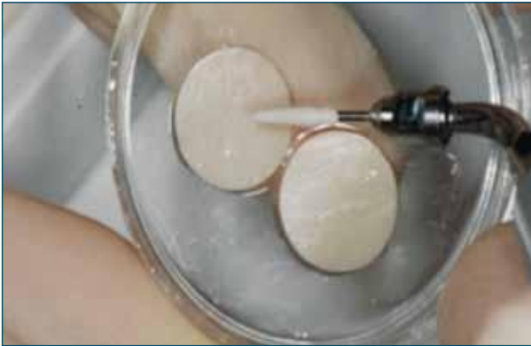
Fig. 4 The samples of Group A1 were treated with a Peek tip (EMS) with a 5" time protocol with horizontal movements.
